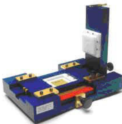
Figure 4-1: Altair BGA Fixture Used for TDR Measurement
